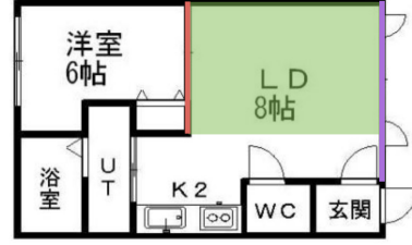
Figure 9: A floorplan example where kitchen and living room appear in the same closed polygon. A pair of facing walls (red line and purple line) with the same room label (e.g., living room) determines that pixels colored with green belong to living room.
