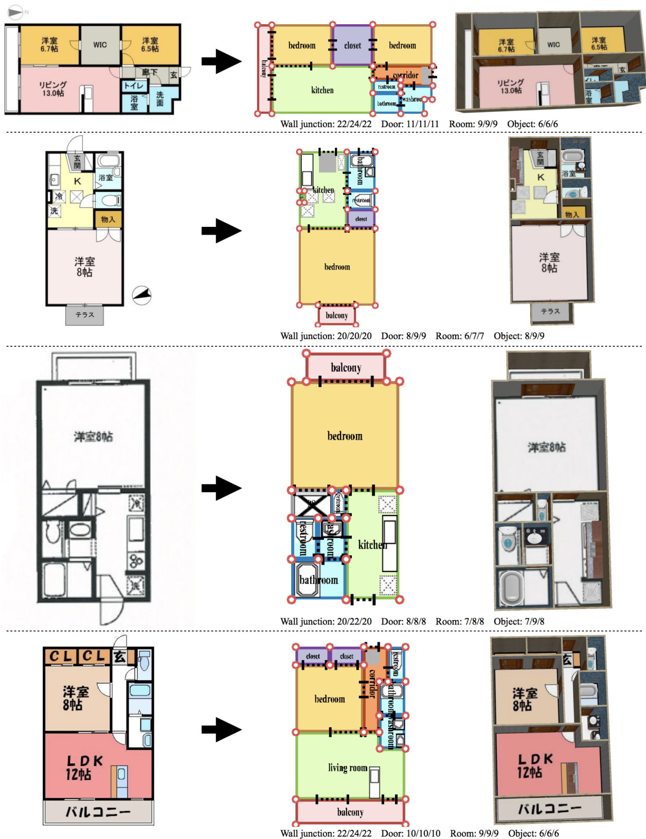
Figure 1: Additional experimental results on test images in our database. The three numbers indicate the same statistics as in the main paper: 22/23/24 mean that there are 23 correct predictions to make, where our algorithm makes 24 predictions and collected 22 correct ones.
