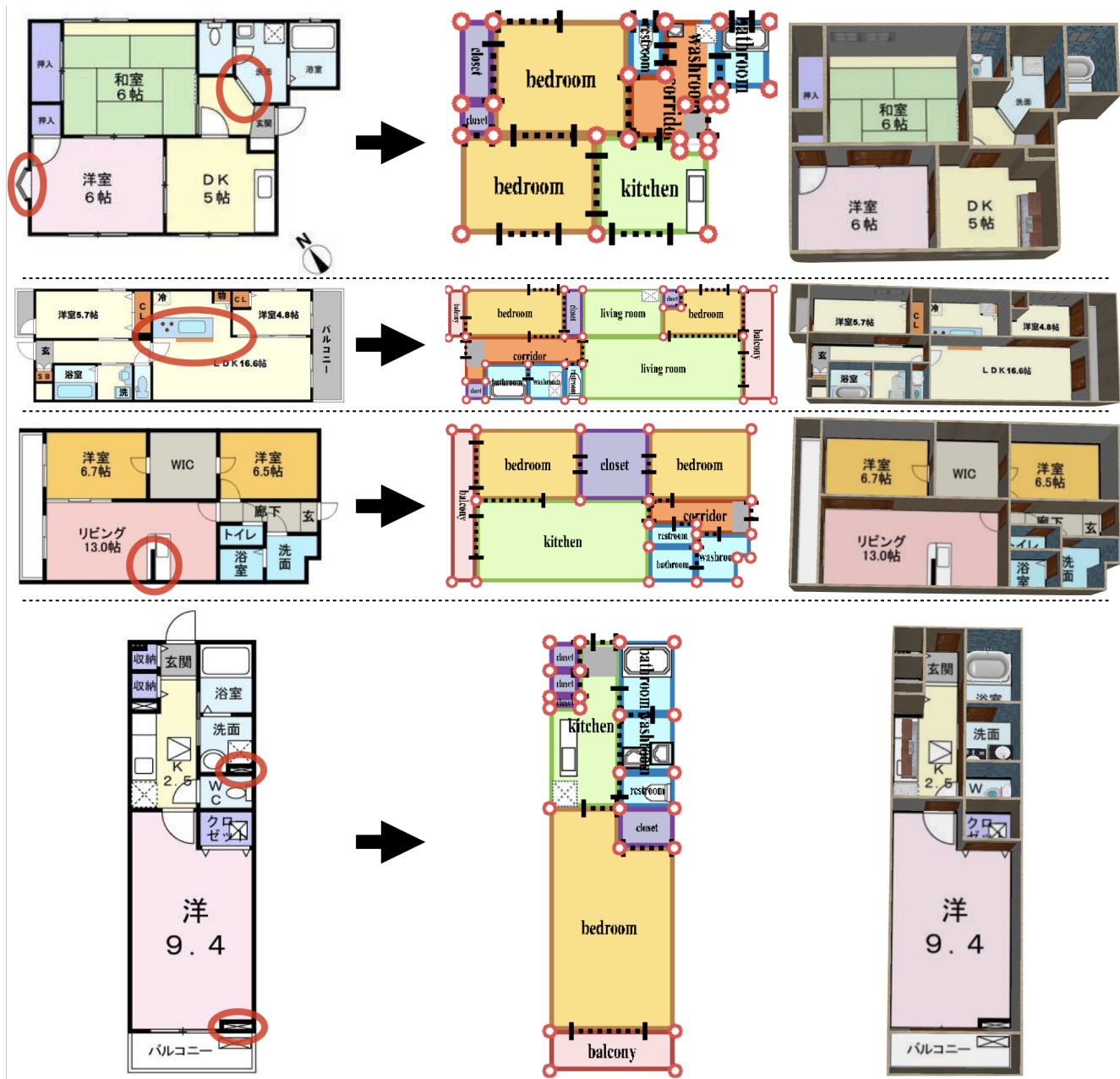
Figure 7: Typical failure cases. Relying on Manhattan assumption, our method is unable to detect walls which are neither horizontal nor vertical as shown in the first example. This is the major limitation of our method, which could be addressed by adding a special wall junction type. In the second example, our method puts a wall which does not exist. In some cases, our method misses I-junctions as shown in the third example and detailed wall structure as shown in the fourth example.
