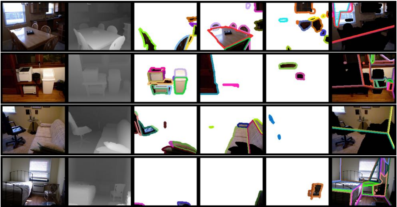
Figure 6. Typical failure cases: (1) When there are many objects in a scene, our method might produce many small surfaces which fail to represent objects in a meaningful way. (2) Our method is capable of capturing most background structures accurately but may fail when the background is complex and contains windows, opening door or large free space. (3) Our method sometimes fails to capture small objects accurately, for example, the bottle on the table and the foot of the chair. (4) In some cases, our method produces many unnecessary surfaces due to the lack of balance between the data term and the MDL term.
